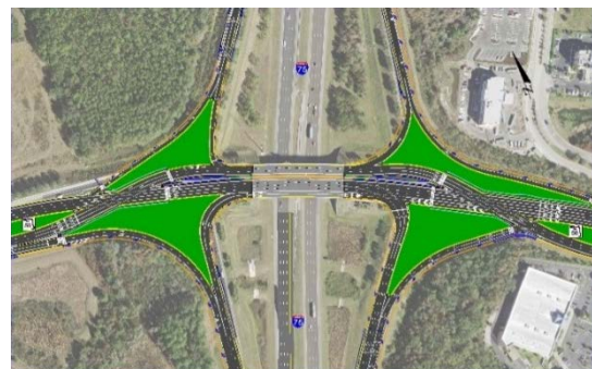
FDOT Diverging Diamond Interchange currently under construction at SR-56 and I-75.
